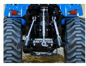
**Durability And Capacity** Heavy-Duty Frame And Lift Cylinders Enable 970 lbs. Of Three-Point Lift Capacity
