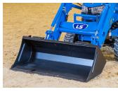
High Capacity Loader 2 Large Diameter Lift And 2 Large Diameter Curl Cylinders Enable 1,007 lbs. Lift Capacity
