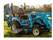
60 Inch Mower Deck Heavy-Duty Mower Deck Provides An Excellent Cut And Makes Use Of The Standard Mid-PTO
