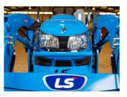
Standard Factory Grille Guard W/Loader Full Length Grille Guard **Protects Body Panels** And Radiator
